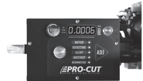
DRO computer compensated for lateral run-out to 0.0006" and ready to cut.
